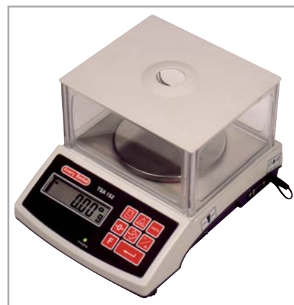
Draught shield available as standard with all models.
